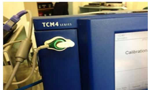
Press the "calibrate" button on the screen of the TCC4 to start the calibration gas flowing to the electrode.
