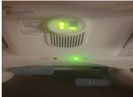
Picture 1. Lights on shuttle indicating battery charge
